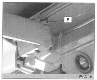
1º Tighten the grub screw (E) to raise the elbow of the arm, and unscrew it to lower.
