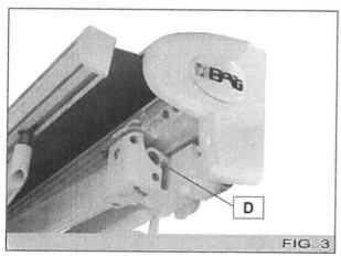
4 once you reach the desired inclination, fasten the awning in position by tightening the screw (D) using a 3 mm Allen wrench.
