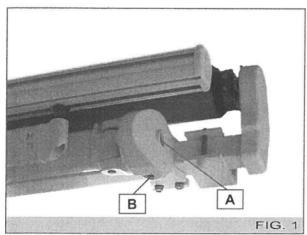
1 Loosen the screw (A) using a 10 mm Allen wrench.
